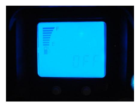
Here, use the right button to toggle this display "OFF" as there is no sending unit on the MadAss 125. Pressing the left button should save the settings and return the speedo to normal display mode.
