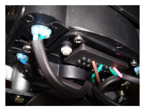
Press and hold this button for about 5 seconds, until the MPH/KPH label starts blinking. The unit is now in program mode.
