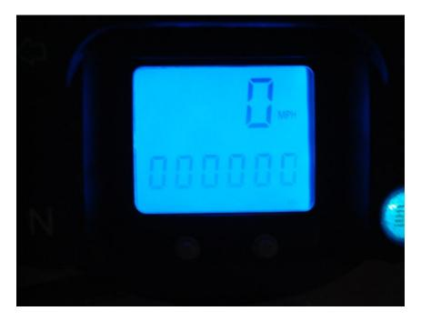
Make sure the digits are all set to "0" values using the same method as for the wheel diameter. Once you advance past the last digit on this screen, you will see the fuel gauge view screen as below:
