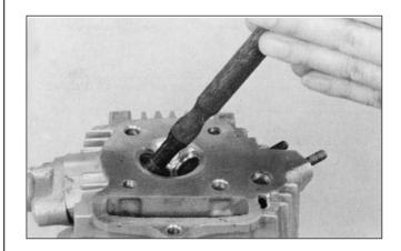
If the contact area is too high on the valve, the seat must be lowered using a 32 degree flat cutter.
