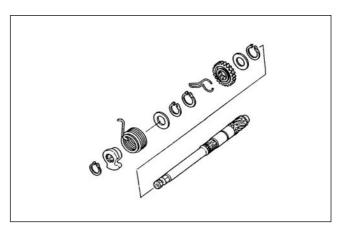
Install the kick starter assembly into the left crankcase by aligning the friction spring with the groove in the crankcase as shown.
