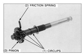
Check the disassembled parts for damage and excessive wear and replace them if necessary.
