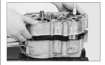
Remove the gasket and dowel pins.
