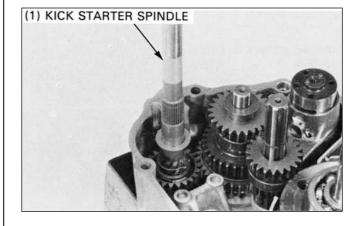
Remove the circlips and remove the kick starter pinion and friction spring.
