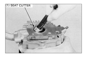
Use a 45 degree cutter to remove any roughness or irregularities from the seat.
