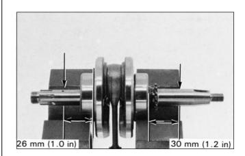
Turn the outer race of the crankshaft bearing with finger. The outer race should turn smoothly and quietly.
