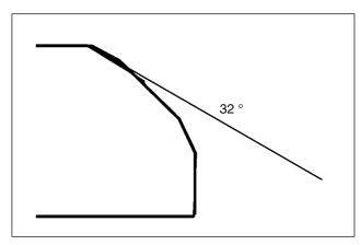
Using 60 degree cutter, remove the bottom 1/4 of the old seat. Remove the cutter and inspect the area you have just removed.
