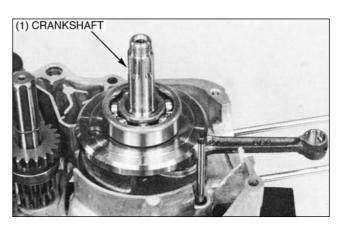
Measure the connecting rod big end side clearance.
