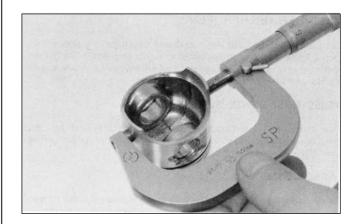
Measure the piston pin bore I.D. in two directions at right angles to each other.
