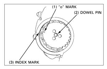
Tighten the cam sprocket bolts.
