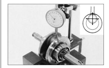
Place the crankshaft on a stand or V-blocks and measure the runout using a dial indicator.
