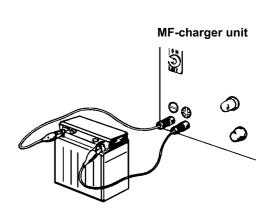
Now check the battery voltage using a volt meter; if the voltage is **lower than 12.5 volt**, the battery must **be recharged** by means of an MF charger unit.
