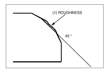
Using 32 degree cutter, remove 1 /4 of the existing valve seat material.
