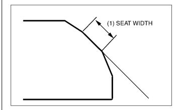
Apply a thin coating of Prussian Blue to the valve seat. Press the valve through the valve guide and onto the seat to make a clear pattern.
