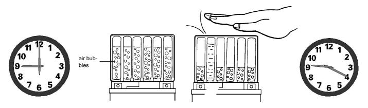
Insert the acid pack into the filler opening of the battery and allow the acid to run into the battery (keep the acid pack in this position for at least **20 minutes**).
