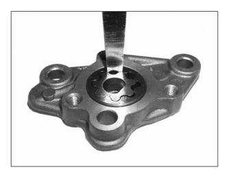
Measure the pump body clearance.
