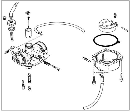
Clear all Jets and carburetor openings with compressed air.
