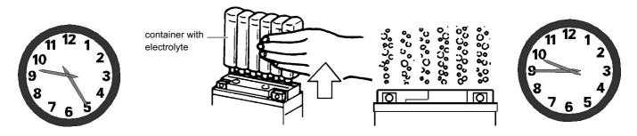
Remove the acid pack from the battery and allow the battery to de-gas for another 20 minutes.
