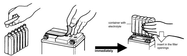
Pull the shut-off plug of the battery from the acid pack and remove the aluminium foil used to seal the battery (once the aluminium foil has been removed, the battery must be **filled immediately**!)
