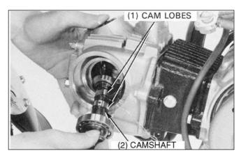
Install the dowel pin into the camshaft.
